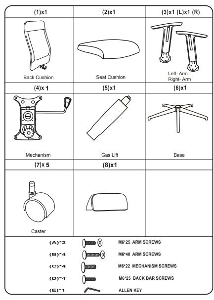
It is important to assemble all parts so that the directional "Arrows" point in the same direction. Make certain that all screws are FULLY tightened before using the chair. Each month, check all screws and tighten any that may have loosened.
